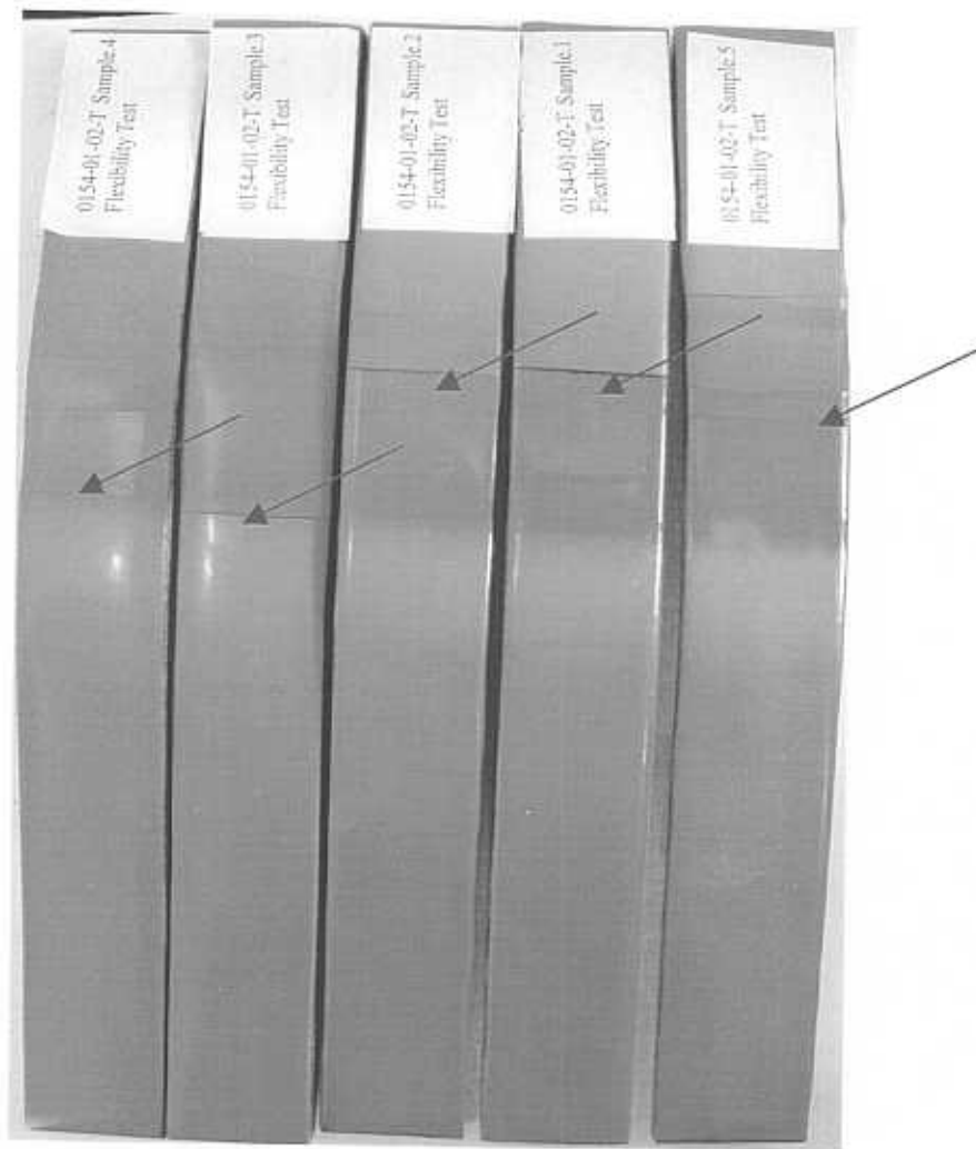
Figure 1. Post-Test Overview – Flexibility Test, 21°C/70°F
