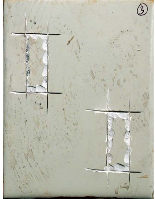
Test Panel Coated and Cured at 21°C/70°F
