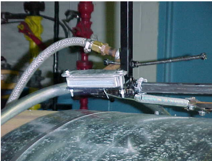
Fig 1 Burner used for Flame Treatment
