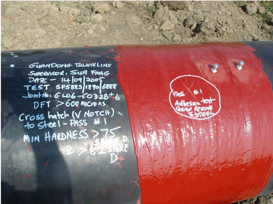
Figure 4. LPE liquid on 3LPE girth weld – BP's Quandong LNG Dapeng Project China
